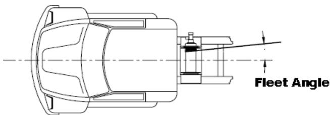
The fleet angle should be kept as small as possible to insure proper spooling and to maximise cable and winch life. To promote even cable spooling, keep the fleet angle below three degrees. Never pull directly against the flange of the winch cable drum as this may cause the cable or the winch to break.
